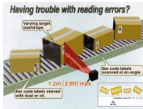
Fig. 97 Bar-Code Reading (Keyence Corporation of America)
