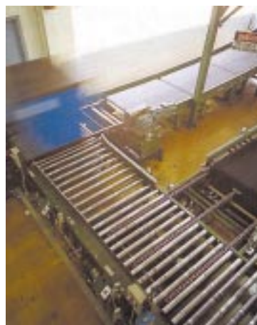
Fig. 115 Right Angle Transfer (Rapistan)
