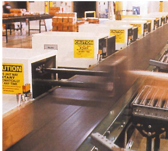
Fig. 109 Air Operated Pusher (Rapistan)
